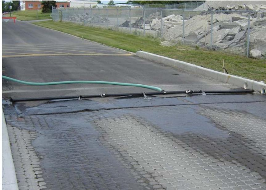
**Figure 3-6: Field Runoff Application Device**
