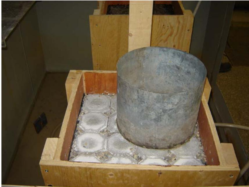
**Figure 3-28: Ring Infiltration Measurement (shown with ground silica sediment on the Eco-Stone<sup>®</sup> model)**
