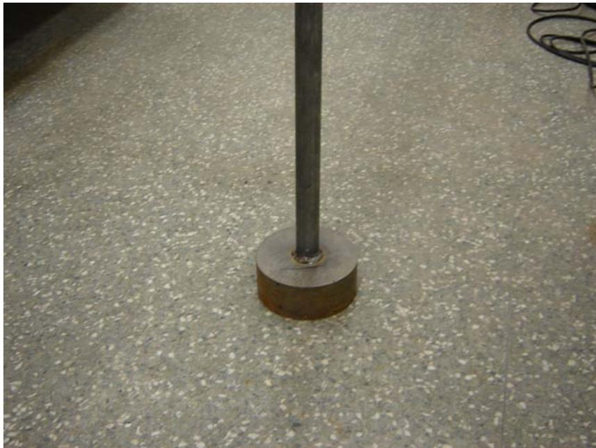
**Figure 3-10: Aggregate Compactor**
