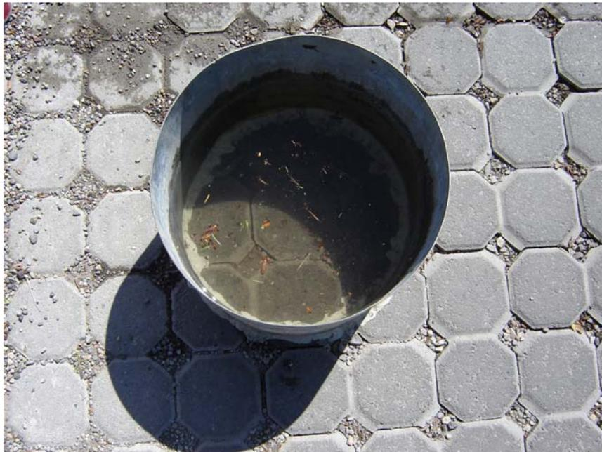
**Figure 3-24: Ring Infiltrimeter Sealed With Plumber's Putty**
