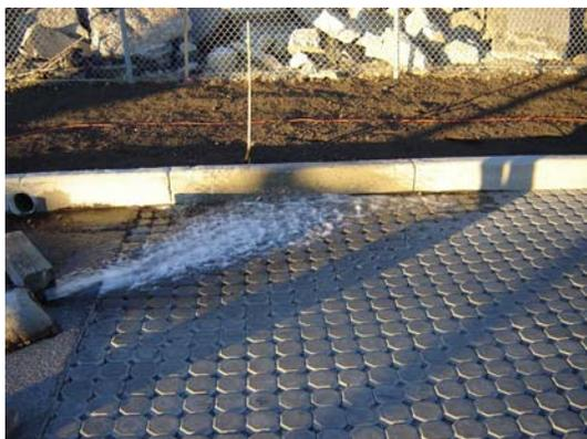
**Figure 4-7: Initial Surface Infiltration Capacity of the Eco-Stone<sup>®</sup> at Currie Barracks, November 24, 2006 (8 L/s Application Rate)**
