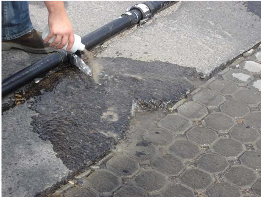
**Figure 3-18: Sediment Application at Currie Barracks**
