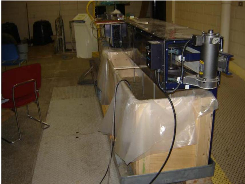
**Figure 3-12: Laboratory Sand Slurry Mixing Tank**
