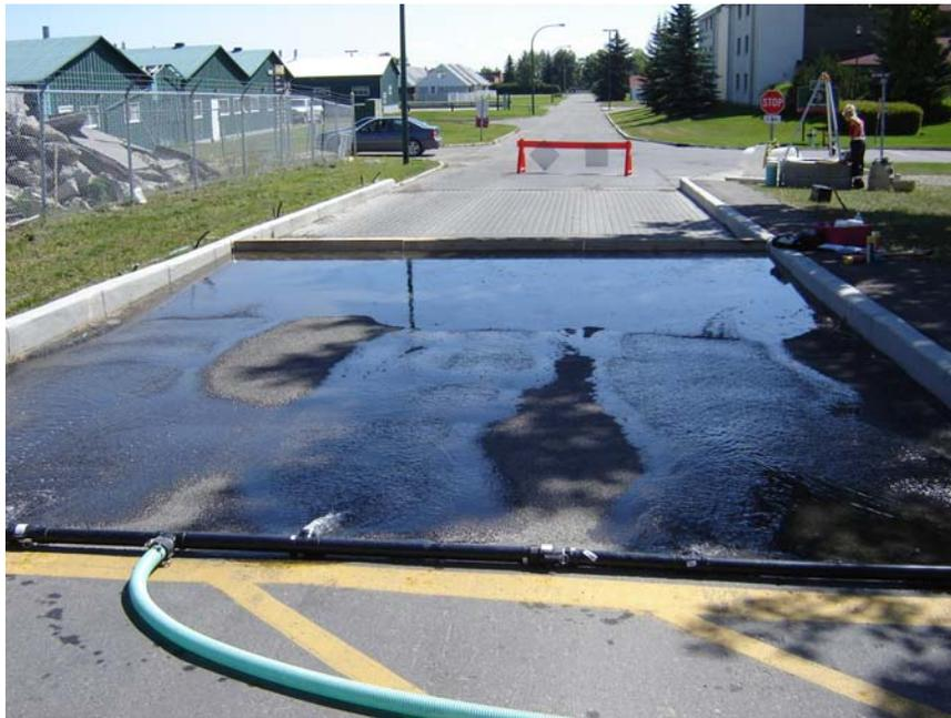
**Figure 3-19: Typical Simulated Runoff Experiment (shown for porous asphalt)**
