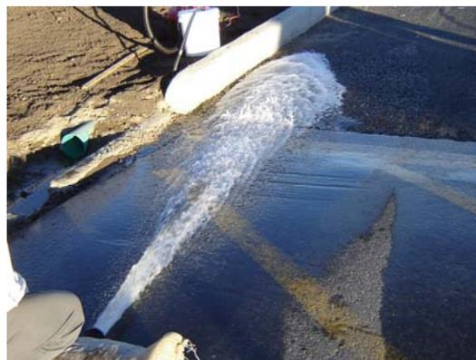
**Figure 4-8: Initial Surface Infiltration Capacity of the Porous Asphalt at Currie Barracks, November 24, 2006 (8 L/s Application Rate)**
