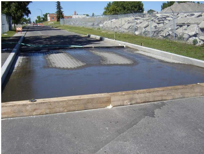
**Figure 3-20: Typical Simulated Runoff Experiment (shown for Eco-Stone®)**
