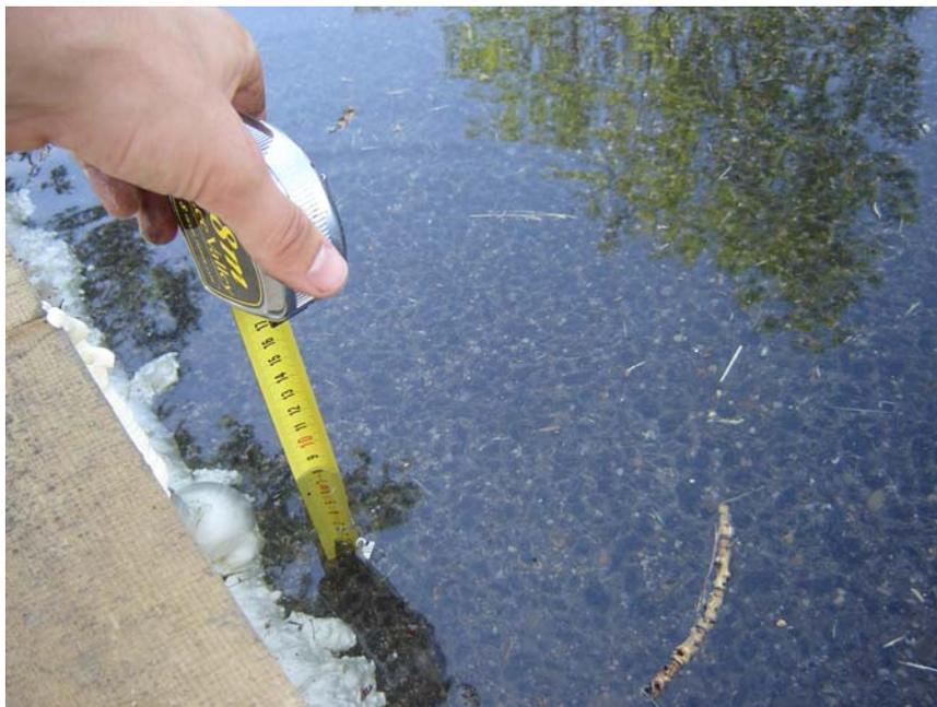
**Figure 3-22: Measuring Maximum Ponding Height**
